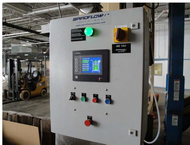
Bulk bag filler gain-in-weight control panel
