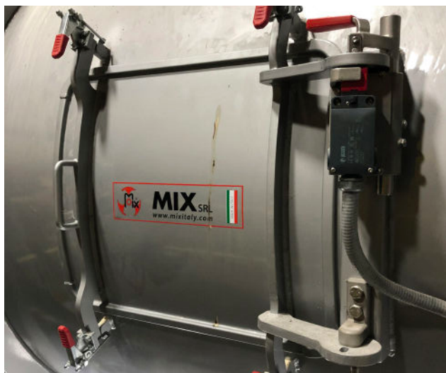
The heavy-duty, interlocked door on the front of the MIXSYS mixer allows for safe operator access.
