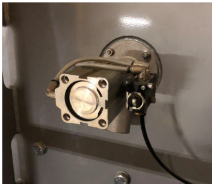
An automatic sampler allows samples to be taken from inside the mixer without the need to open the mixer or stop the system.
