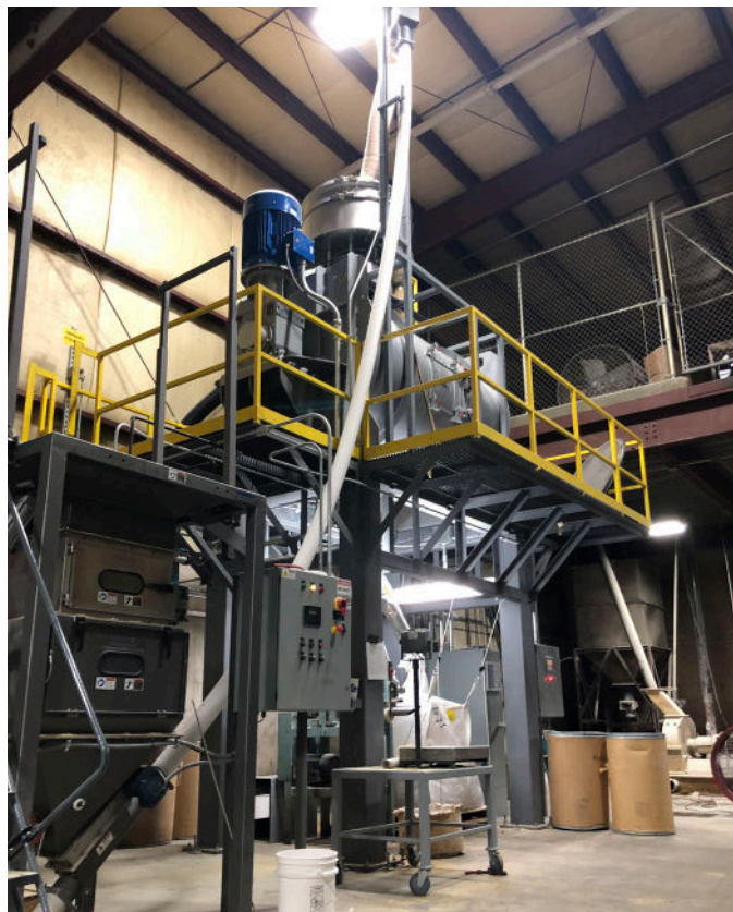
The Spiroflow T2 bulk bag unloader with an integral sack tip station and FSC412-B flexible screw conveyor delivers raw materials to the screener on the mezzanine level above.
