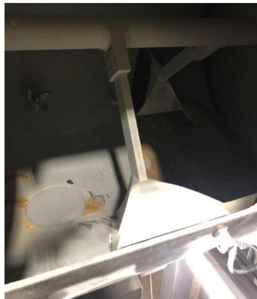
Plow-shaped mixing tools inside the MIXSYS Ploughshare mixer carefully and thoroughly mix high volumes of materials with different particle sizes with minimal product degradation.
