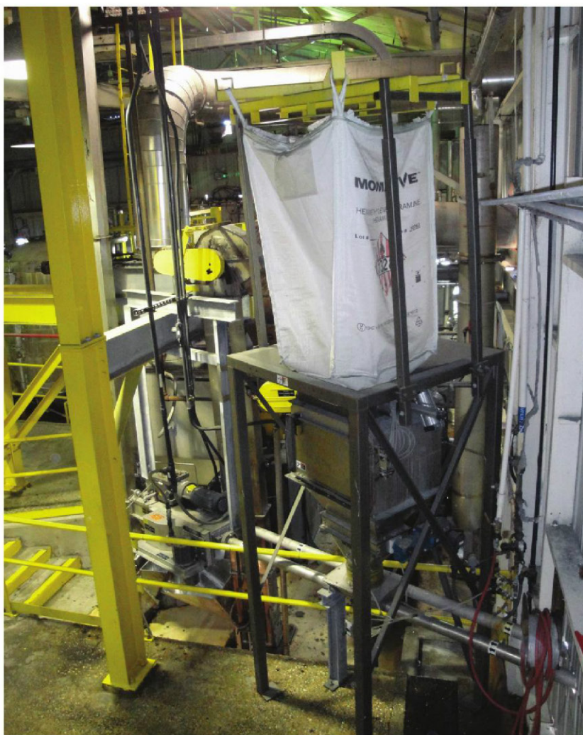
The bulk bag unloader allows for the safe and accurate release of hexamine into the conveying system.
